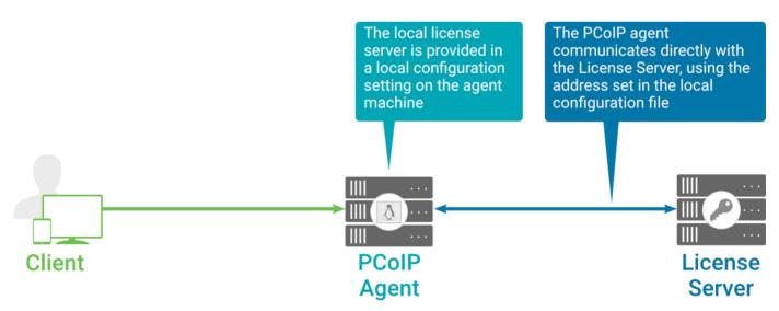
Local license validation using a Remote Workstation Card Agent for Linux and a direct (unbrokered) connection
